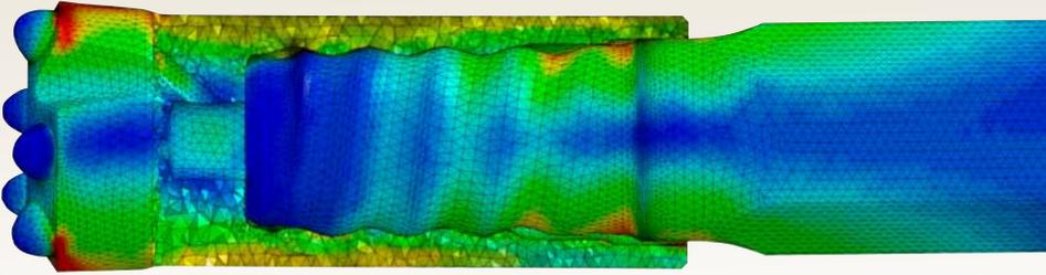
Advanced analysis have been used to simulate and locate critical bending stresses of various designs to arrive at an optimally dimensioned rod / bit connection.
