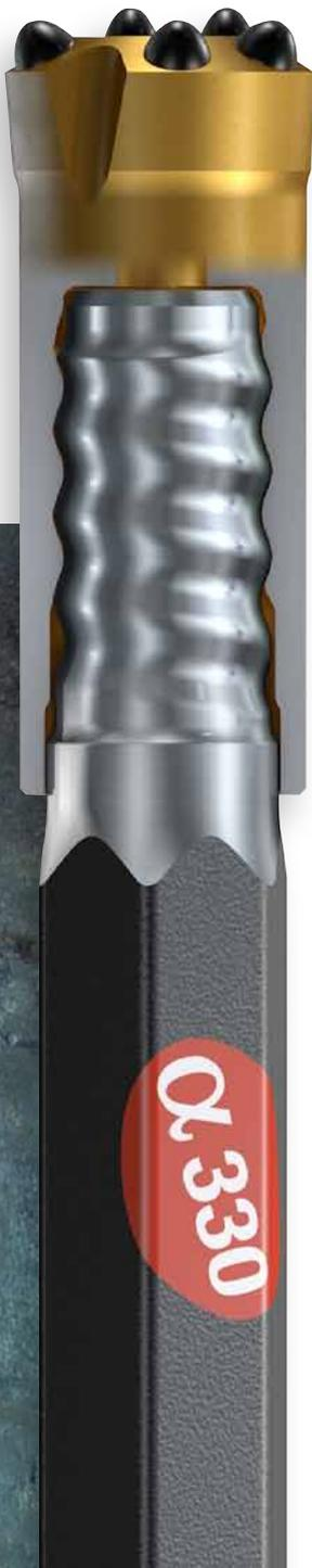
**A snug interface at this crucial point at the rear of the connection greatly improves the rigidity of the joint. The bit skirt covers the thread completely in the Alpha 330 connection, no part of the thread itself is exposed to sandblasting, reducing the risk of corrosion-fatigue.**
